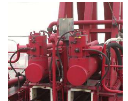
Hydraulic protection against snag
