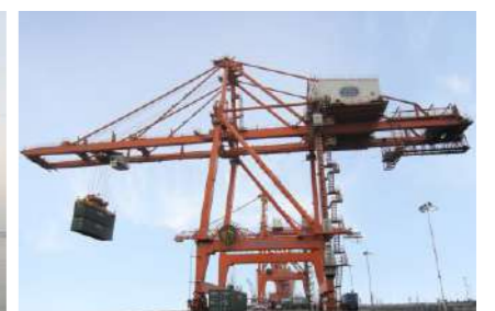
Overload test of the complete crane
